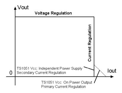
**Output Voltage vs. Output Current**
